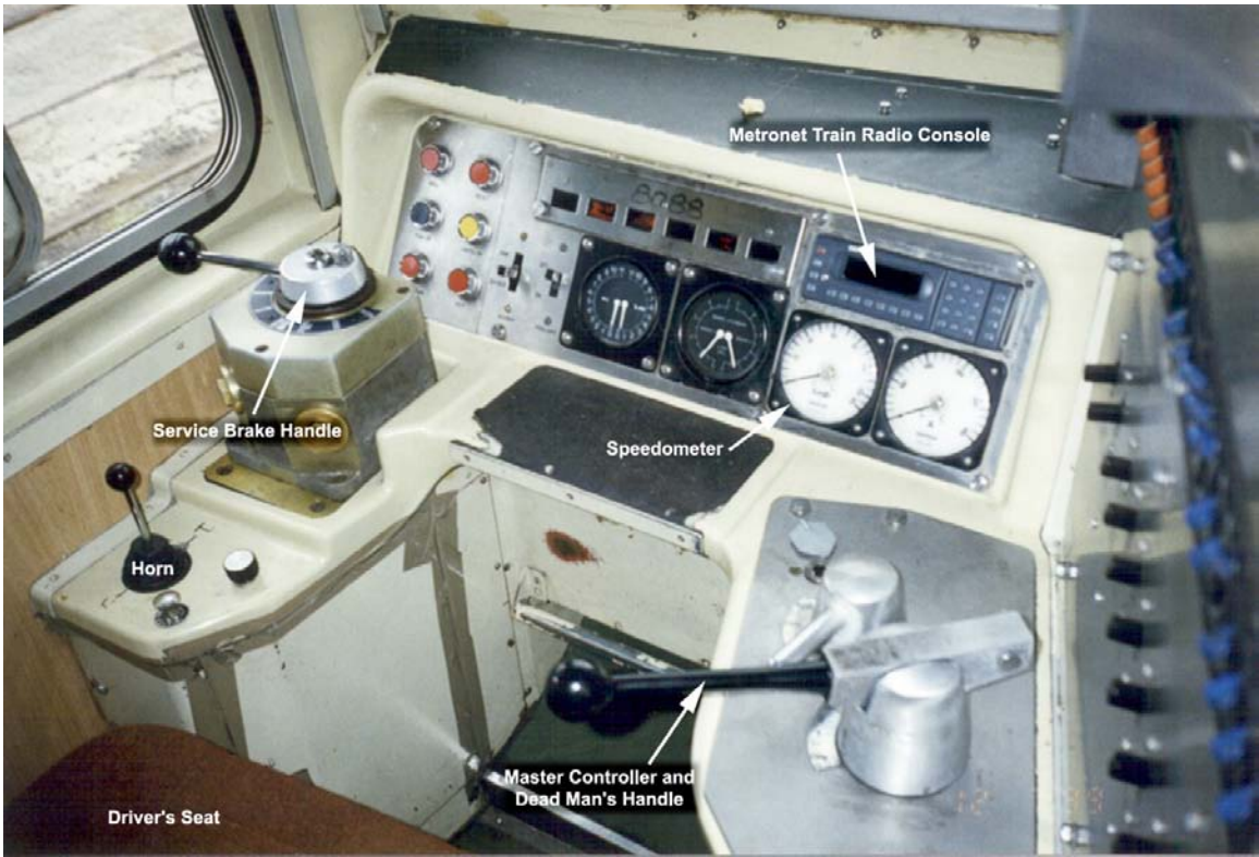
Figure 23 - Driver's compartment of an inter urban train similar to that involved in the accident
