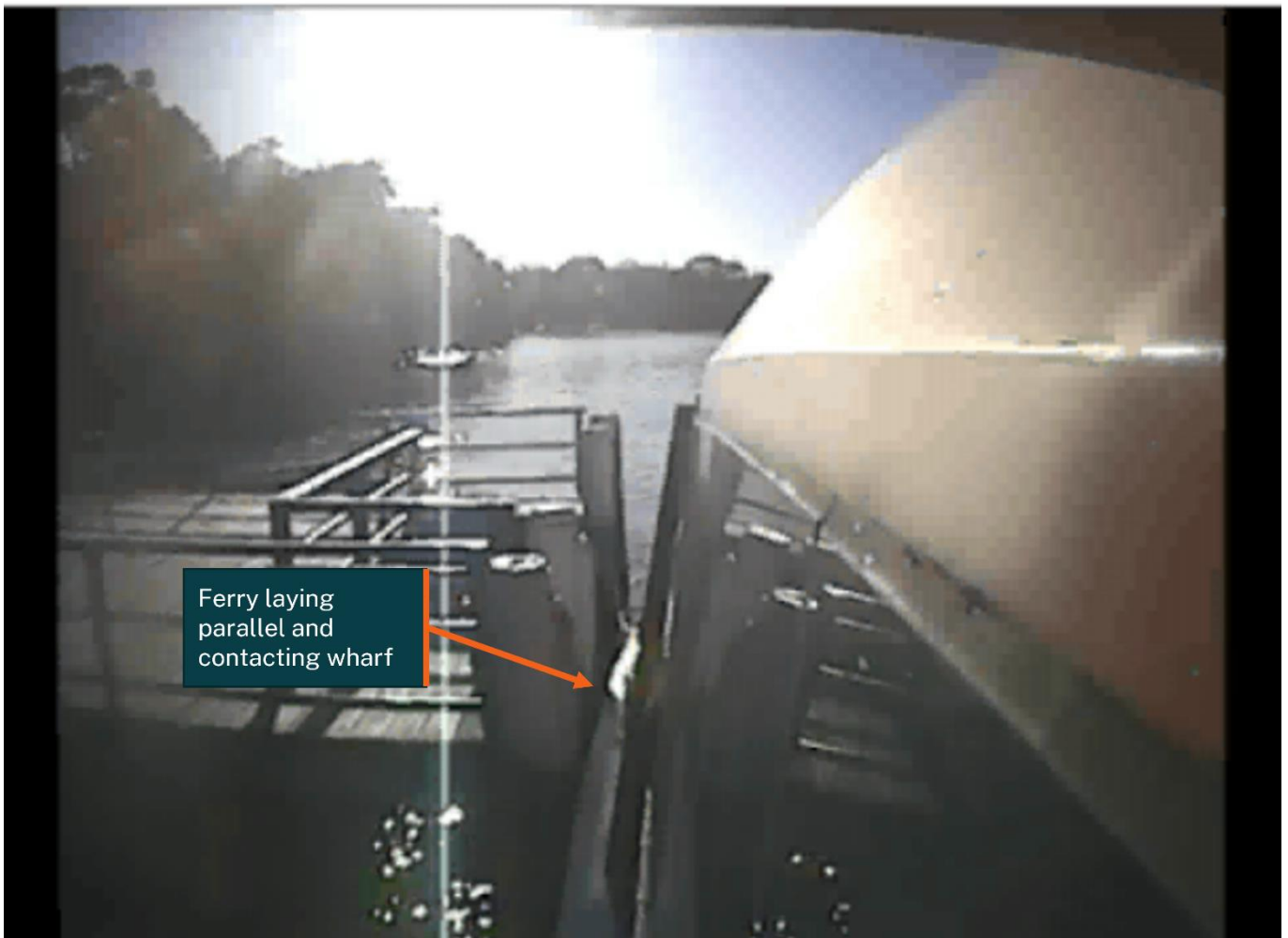
Figure 3: Onboard portside CCTV showing position of vessel alongside the wharf before the incident
