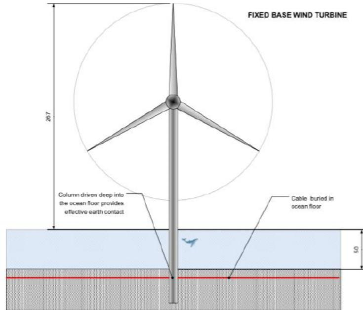
The diagram above is for a fixed base turbine.
