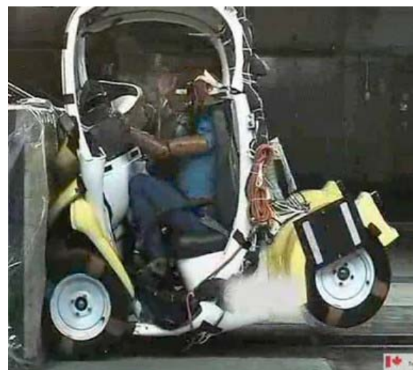
Figure 1. Transport Canada crash test of a car-like quadricycle vehicle (40km/h full frontal)
