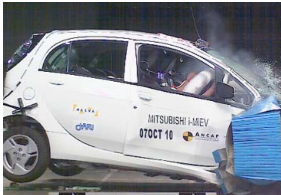
Figure 3. ANCAP crash test of Mitsubishi i-MiEV (64km/h frontal offset)
