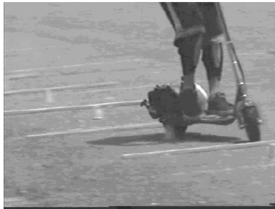
Performance test with obstacles across path
