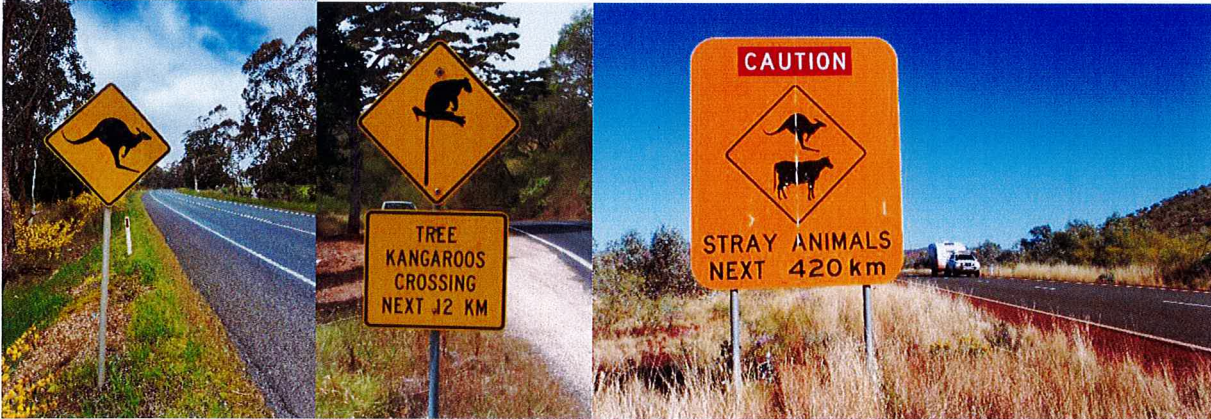
Figure 4.10. Examples of static wildlife warning signs with increasing (from left to right) levels of information for motorists. Photos by Rodney van der Ree, WSP.
