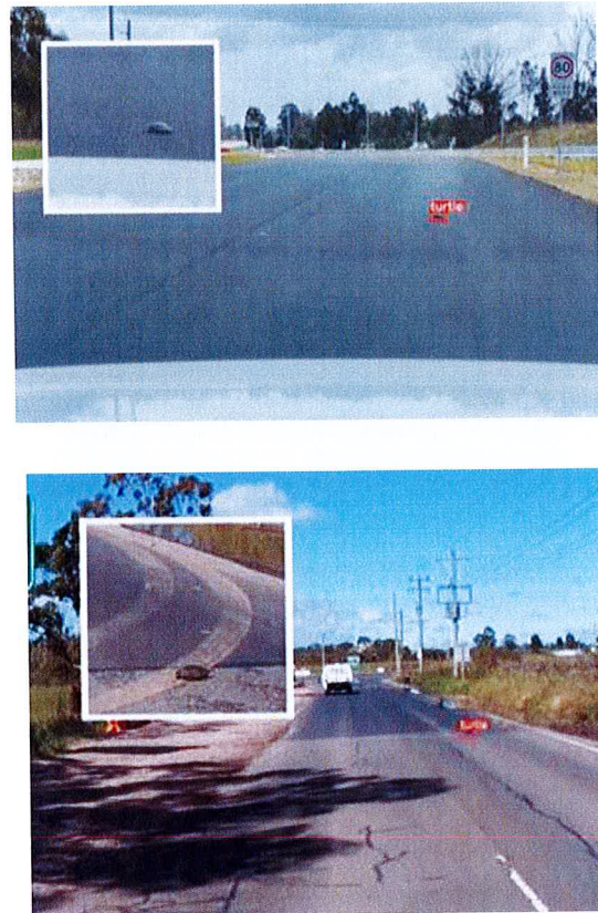
Figure 5.8. Examples of 'TurtleSAT' vehicle-mounted animal detection system imagery. Source: Jim Steen, TfNSW
