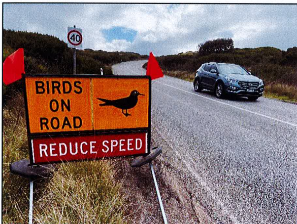
Figure 4.12 Enhanced roadside wildlife warning sign, specific to the Short-tailed Shearwater, installed for a few weeks per year at Phillip Island, Victoria, Australia.
