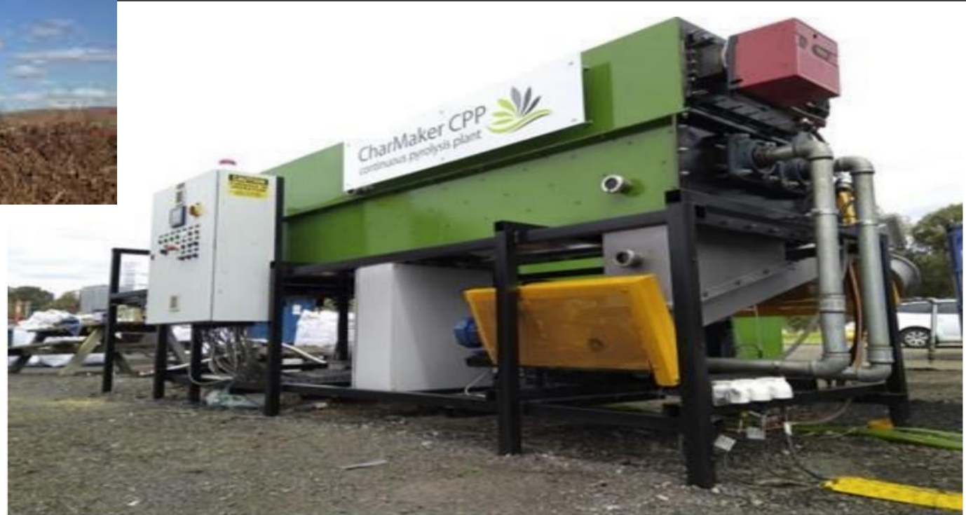
FIGURE 13 CHARMAKER CONTINUOUS TECHNOLOGY DESIGNED AND BUILT BY EARTH SYSTEMS PROCESSES A RANGE OF FEEDSTOCKS.
