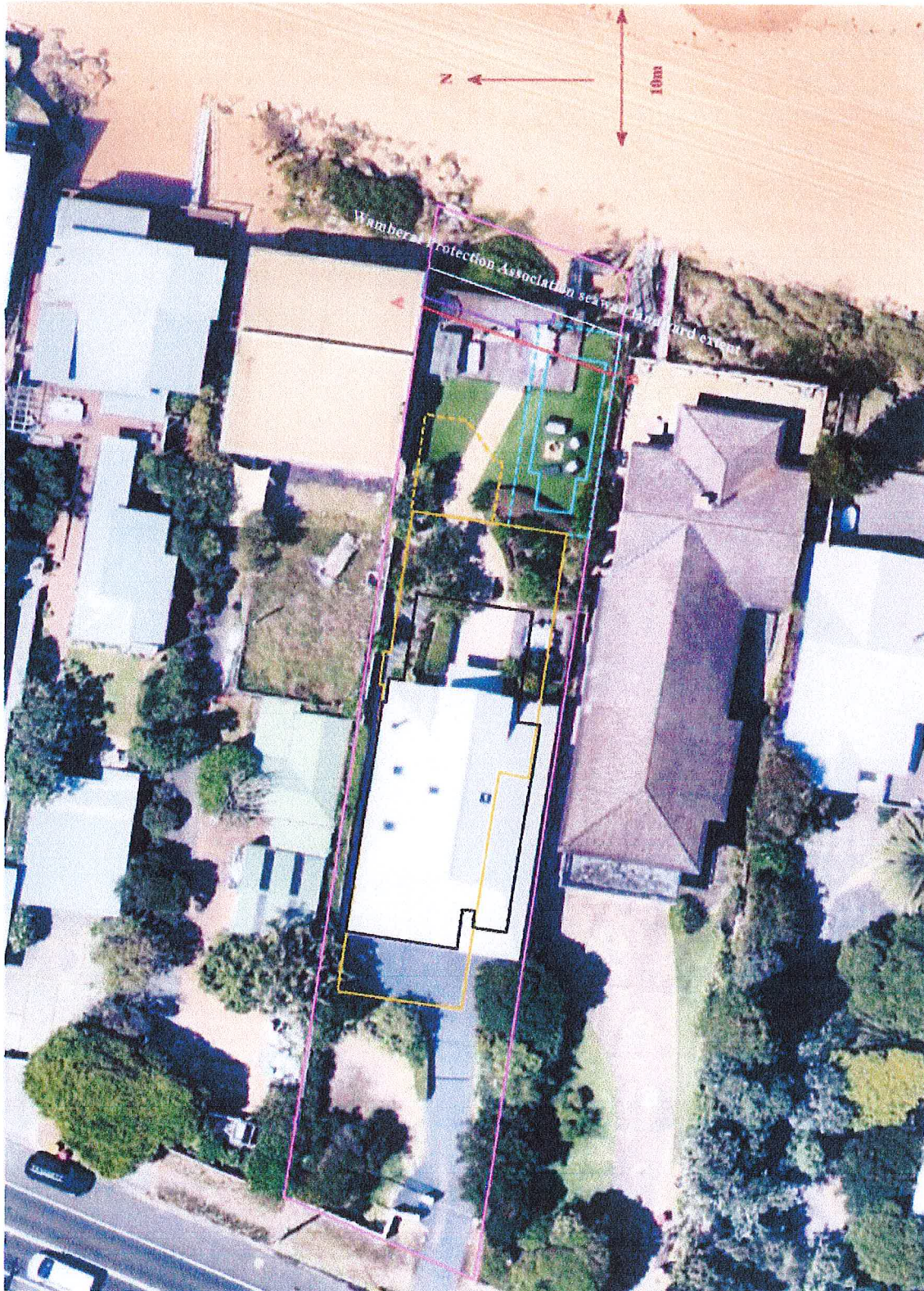
Figure 1: Landward edge of proposed WPA seawall in white and 3m setback from this in red, with proposed upper ground floor outline in yellow (terrace dashed), lower ground level in black, pool and spa in cyan (pool court dashed) and firepit court in purple (aerial image taken 14 March 2024)
