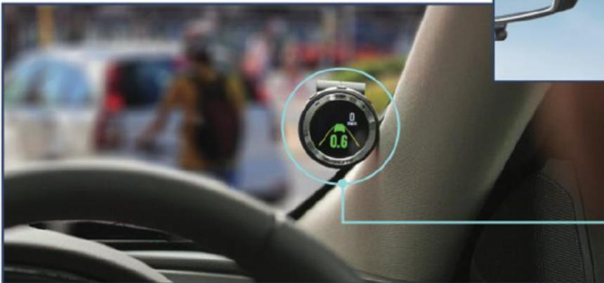
The EyeWatch™ display for visual alerts, mounted in the bottom corner of the windshield
