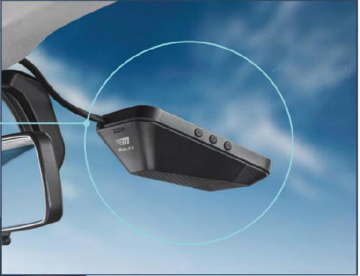
The camera unit containing the camera, EyeQ® chip, and speaker, mounted on the inside of the windshield behind the rearview mirror
